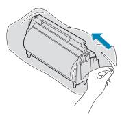
4 Remove the paper covering on the imaging unit by removing the tape under the handle of the imaging unit.
